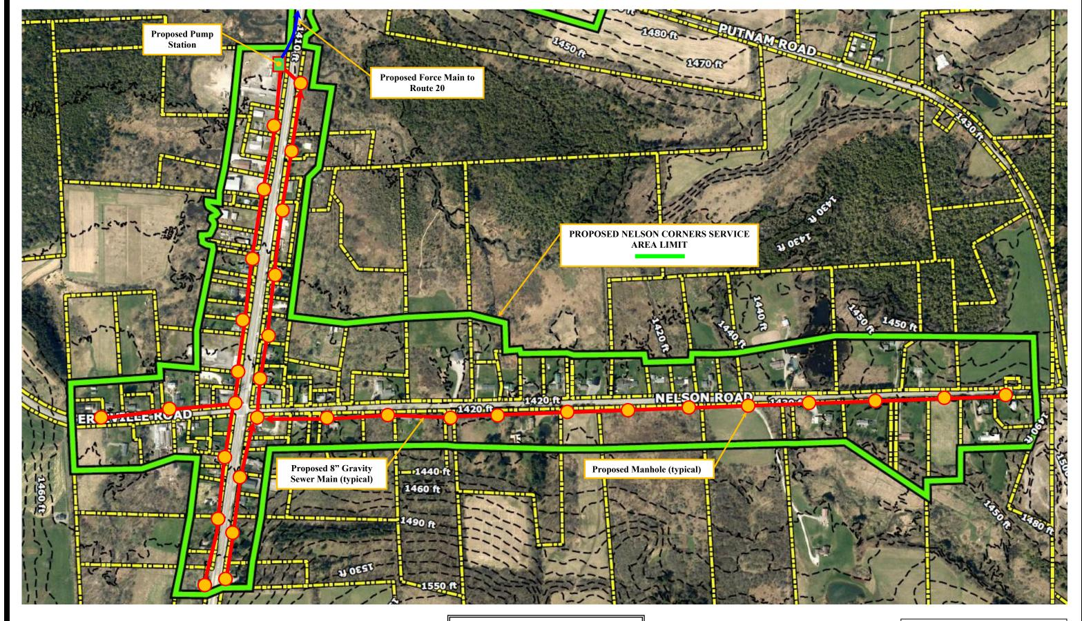
POTENTIAL NELSON CORNERS SERVICE AREA LAYOUT 33 Manholes 1 Pump Station 11,900 Feet of 8" Gravity Sewer Main
